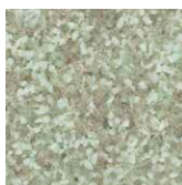
CERAMIC Ceramic grain and monocrystal aluminium oxide
